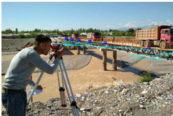
Fig. 2. Scheme of leveling results – Phase I (without load, before testing)
