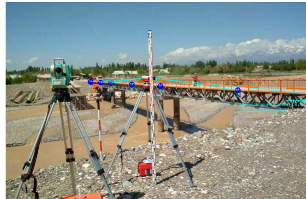
Fig. 3. Scheme of leveling results – Phase II (load P = 45 tons)
